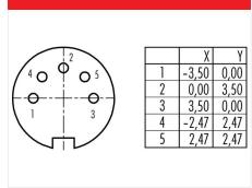
Contact arrangement (Plug-in side)
